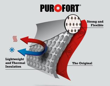
Purofort® is the unique Dunlop® material with millions of evenly distributed air pockets making it lightweight and thermally insulating plus a cross-linked structure that provides flexibility and strength.
